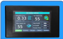
Intuitive Color HMI Display with touch screen interface for various controls along with on screen UV & HEPA life display and USB data logger
